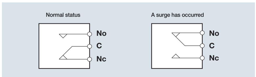
\* During the normal status (NC contact), the device operates normally. However, when the internal separator is activated due to the degradation of the product by a surge, the AL contact will be switched to a No contact.
