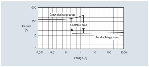
V-1 Characteristics of the discharge tube
