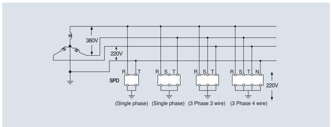
\* The applied voltage is 380V between phases, but as SPD sets the ground, it becomes 220V based on the ground potential. SPD should be selected and installed in consideration of Maximum continuous operating voltage (MCOV) and the voltage protection level (Up).
