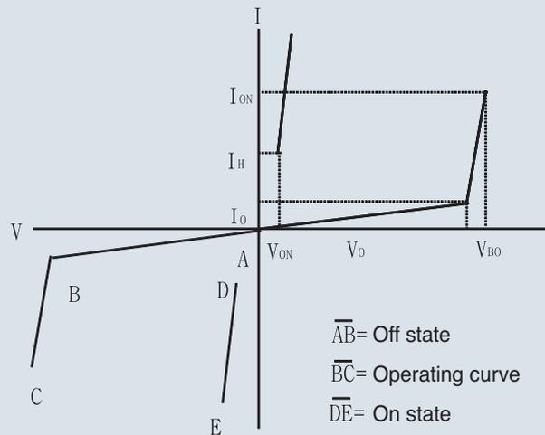
V-1 Characteristics of the silicon restriction element
