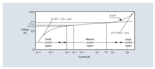
V-1 Characteristics of the Metal Oxide Varistor (MOV)
