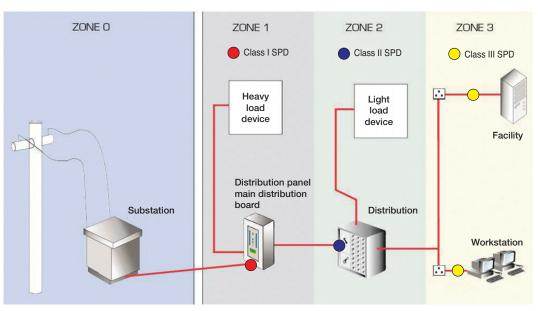
Note) If the heavy load device or light load device is 20m or farther from the SPD installation position in the unshielded vertical wiring distance, the additional protection should be considered.
