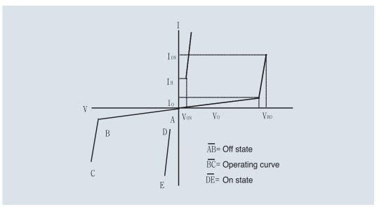
V-1 Characteristics of the silicon restriction element
