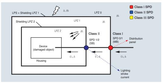
LPMS using the protection of the SPD cooperative with the space shielding object -The device protected well from the conductive surge and from the radiating magnetic field-
